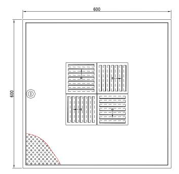
Model PCD diffuser are recommended for heating, ventilating, and cooling. Design for surface mounting in all types of ceiling. Provides a displacement system giving improved air quality and lower temperatures in the occupied zone. The perforated distribution plate provides a constant air distribution over the entire face area without any risk of draught.
